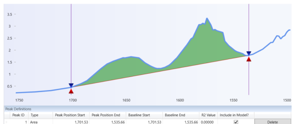
Figure 5. The peak area determination of the vibration spectrum of metformin hydrochloride standard solution in methanol (concentration of 50 mg per mL)
